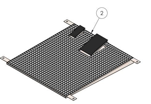
1160 /Floor grid with foot activation for emergency shower and eyewash. Grid dimensions: 1225x1070x25
